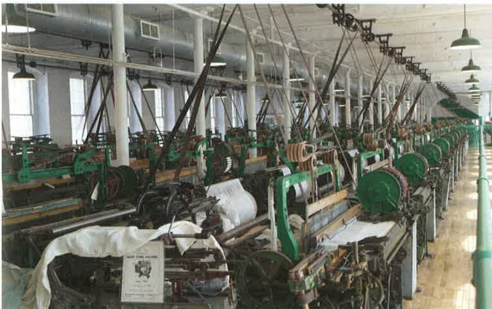
At the start of the Industrial Revolution, factories using specialized machines began to replace hand spinners and weavers in the production of cloth. These old mechanical looms can still be seen in operation at the Boott Cotton Mills Museum in Lowell, Massachusetts.
